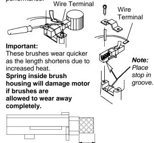
Periodically check the length of the carbon brushes. Replace both carbon brushes when either is less than 3/8" long.
